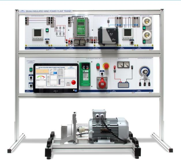
With this equipment, we emulated the behavior of a wind turbine in a practical and didactic way. An electric motor acts as the blades and bush of a wind turbine, dragging a three-phase synchronous generator of permanent magnets, which transforms the mechanical energy transmitted to the shaft into electrical energy at the output.
